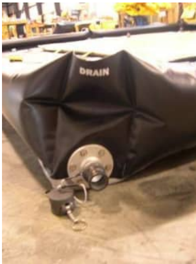
Photo #1: 2”Drain connection
