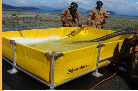
Canflex Collapsible Modular Frame Tanks are foldable tanks for bulk liquid storage. A wide range of special government approved material coated liners are available for these tanks. They can be used in many environments. All seams are constructed with RF welding with a 2.0" electrode. NO GLUE or sewing is used. The resulting seam strength of the welds is equal to or greater than the strength of the parent fabric.
