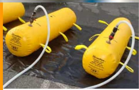
Lifeboat and Davit Test Water Bags are used for evenly distributed load tests. These load test bags come with fill/offload fittings and an automatic relief valve which is activated once the lifeboat bags achieve the desired weight.
