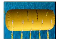
The Canflex **Model (ELB) Pontoon bags** are cylindrically shaped (totally enclosed units) used for supporting loads. These units are equipped with positive venting relief/dump valves mounted along the top. These valves are spring loaded and spring pressure set to automatically open when overpressure.
