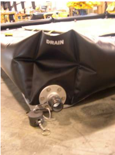
Photo #1: 2”Drain connection
