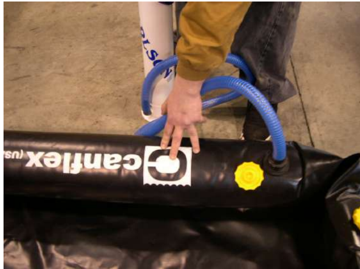
Photo #2: Air tube w/ pump & valves
