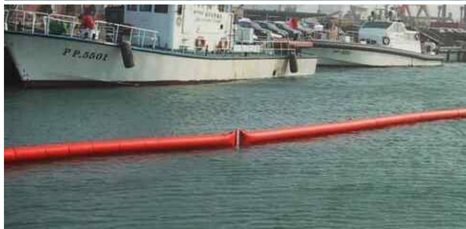
All seams radio-frequency (RF) welded Inflatable buoyancy chamber, full length
