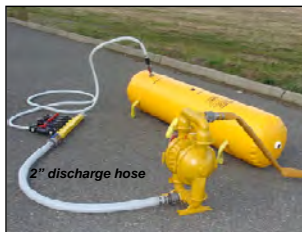
LBB with 1" PVC ball valve with female camlock & 1" hoses
